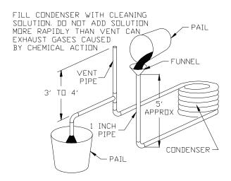
**FIGURE 9 - GRAVITY FLOW METHOD**
